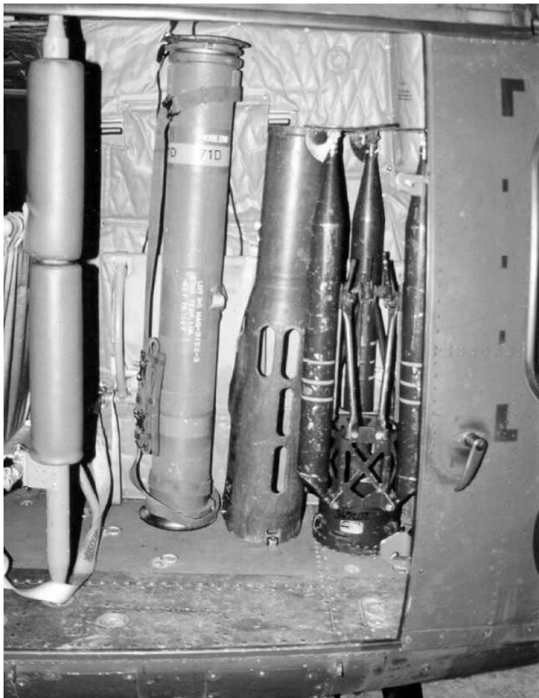
Figure 2-12-1: Stowage of Tripod, Launch Tube and Missile
