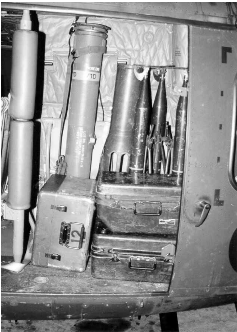
Figure 2-12-2: Stowage of MGS, Collimator and Thermal Sight
