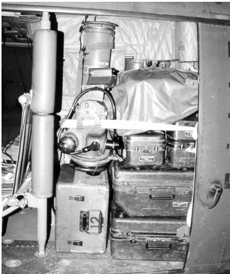
Figure 2-12-4: Stowage of OSS and Securing of Cargo
